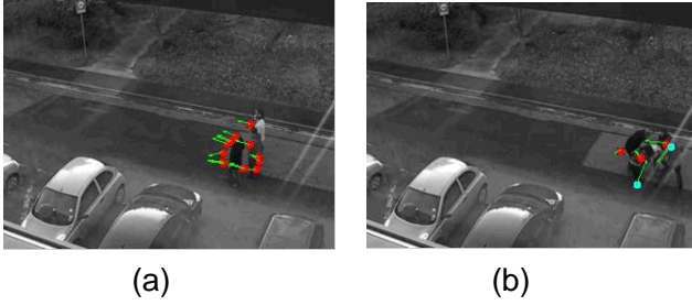
Figure 2. Interaction energy potentials of two sample frames. Green arrow is the velocity; round dot denotes energy values. Red dot shows a low energy value and blue shows a high value.
